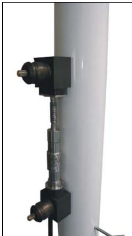
This subsea strain sensor assembly (SSSA) alerts operators to excessive tensile and bending strain along a pipeline at water depths up to 10,000 ft (Fig. 3).
